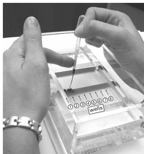
Figure 1. Loading the methyl orange dye sample into the second well of the gel.
