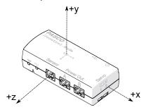
When motionless, the accelerometer measures  $+9.8 \text{ m/s}^2$  when pointing *away* from the ground and  $-9.8 \text{ m/s}^2$  when pointing *towards* the ground. This is useful for determining the //control.Node's orientation. For example, if the y-axis is pointing away from the ground, the **Acceleration - y** measurement reads  $9.8 \text{ m/s}^2$  and the other axes measure 0.
